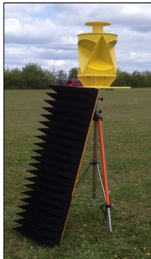
Figure 51: RF absorber
