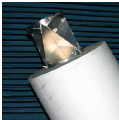
Figure 47: radar reflector without cover
