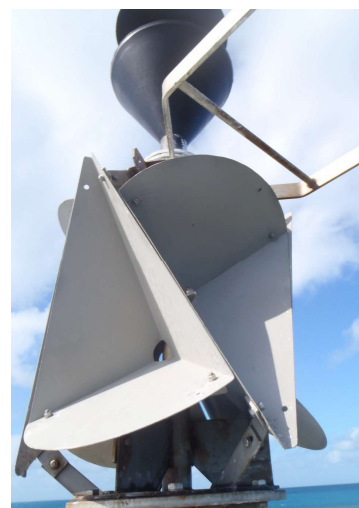
Figure 34: radar reflector consisting of single corner reflectors mounted on a structure
