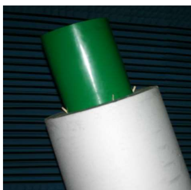
Figure 48: radar reflector with plastic cover
